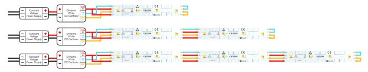
Advantages of this solution are very effective operation and uniform distribution of light. Higher voltage supply is require, when large number of LED modules are connected. If too many LED modules are connected, the voltage value may not meet requirements of SELV. Non-SELV voltage need additional protection. All above connections are examples and may be different from the actual.
