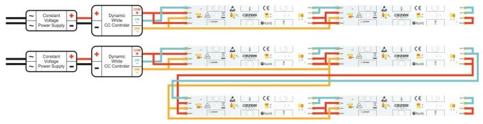
To meet SELV requirements LED modules may be connected with serial-parallel wiring, maximal two LED modules in serial. Advantages of this solution are lower voltage and higher current.
