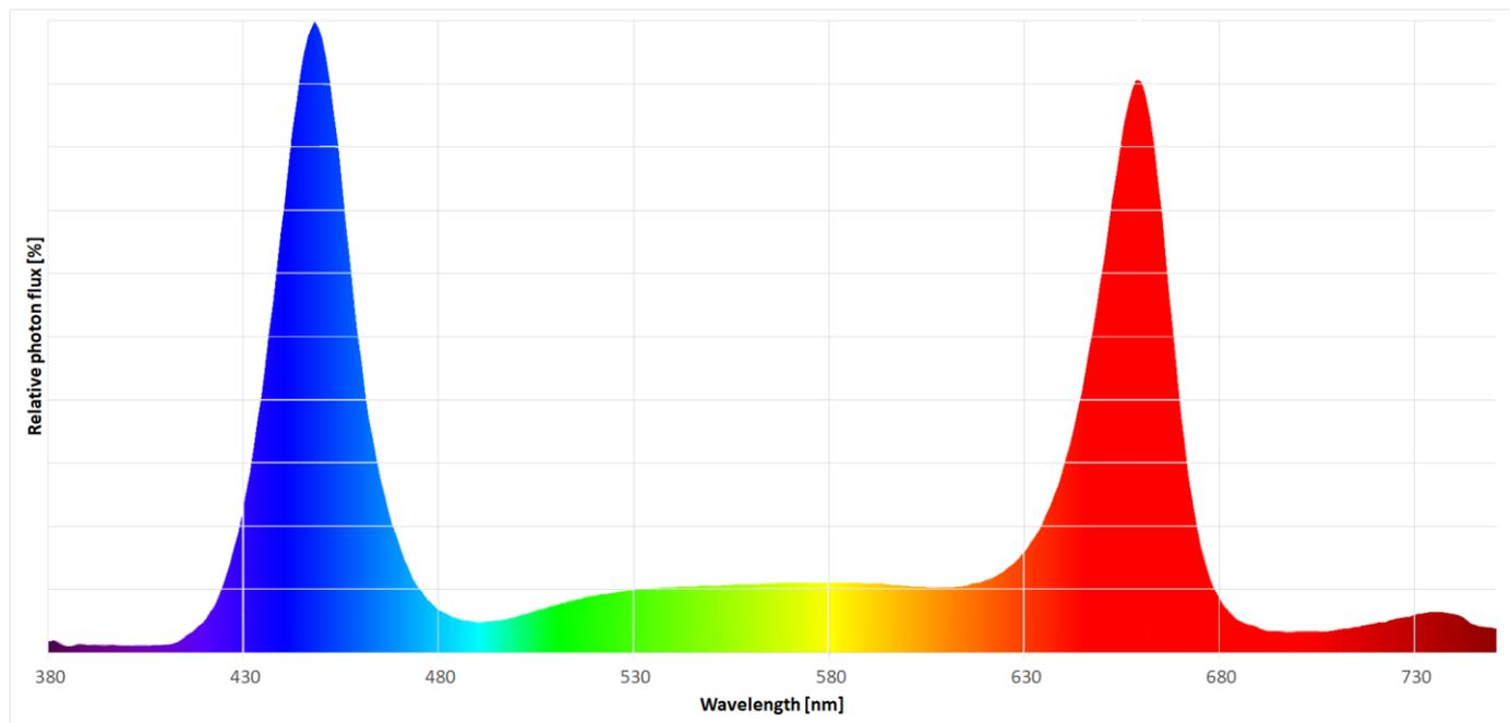
Normalized spectrum graph of the red, far red, blue and white LEDs at 350 mA current. Spectrum can be changed by choosing LEDs and power output.
